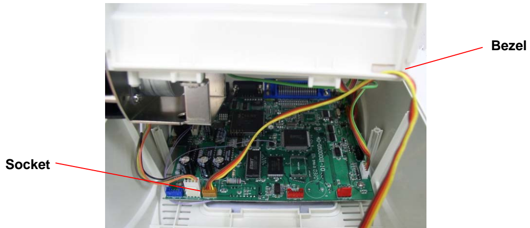
Fig. 16 Cutter module harness arrangement
