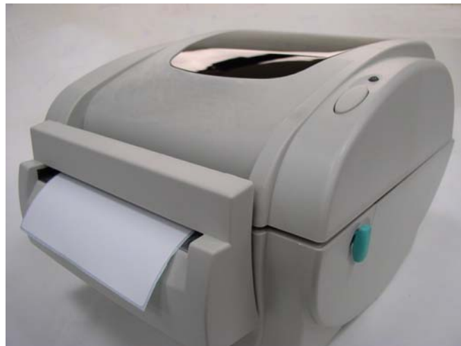
Fig. 19 Media installation in cutter mode completed
