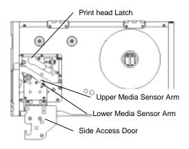
Figure 11 - Print head Latch and Side Access Cover
