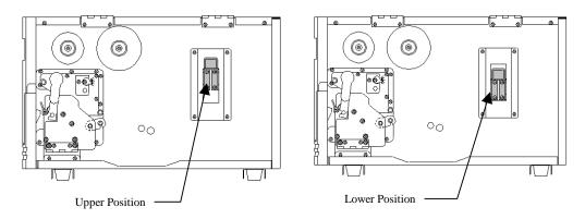
Figure 19 - Media Spindle Location
