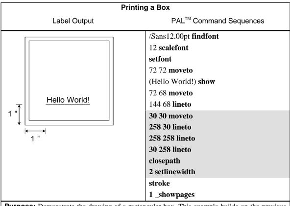
**Purpose:** Demonstrate the drawing of a rectangular box. This example builds on the previous example by drawing a frame around the label. A 4" x 4" (288 points x 288 points) label is used in this example. The frame will be placed within 30 points of the edge of the label.
