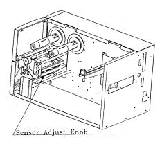
Figure 17 - Media Sensor Adjust Knob
