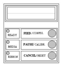
Figure 21 - Fastmark 4000 Series Front Panel
