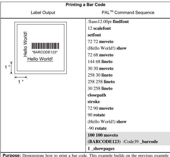
**Purpose:** Demonstrate how to print a bar code. This example builds on the previous example by placing a bar code near the center of the label.
