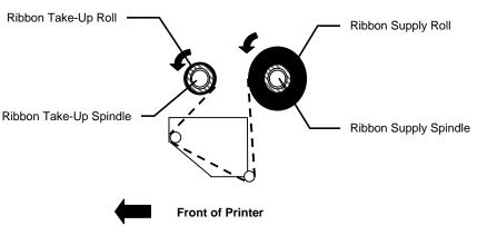
**Figure 13 - Ribbon Routing**
