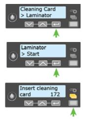
The laminator pulls the cleaning card from the card exit slot into the laminator and moves it back and forth through the L1 and L2 cartridge areas, the card entry area, and the exit rollers several times. If the system has locks, the used card is ejected into the laminator reject tray. If the system does not have locks, the used card is ejected into the laminator output hopper.
