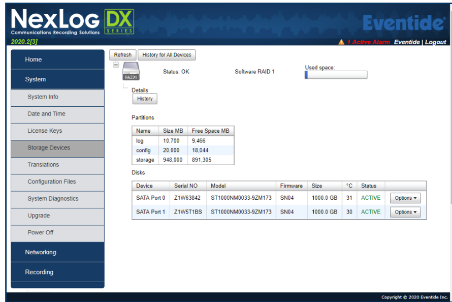
Fig. 7.4 Storage Devices: Hardware RAID-1 Example
