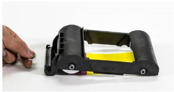
Figure 18 Peeling the protective wrapper
