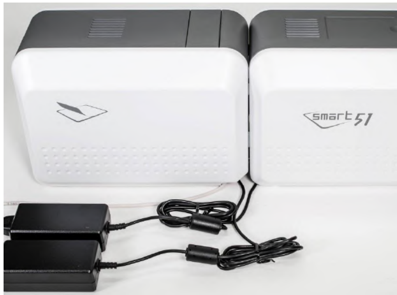
Figure 12 SMART-51L Connection of powers and USB cable - 2
