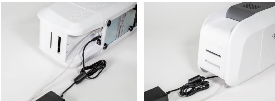
Figure 10 SMART-51D Connection of power and USB cable
