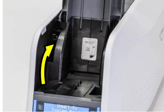
Figure 24 Adjusting the card thickness lever
