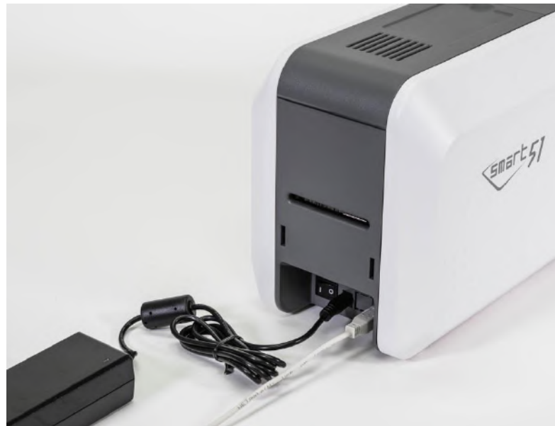
Figure 9 SMART-51S Connection of power and USB cable
