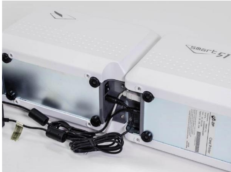
Figure 11 SMART-51L Connection of powers and USB cable - 1
